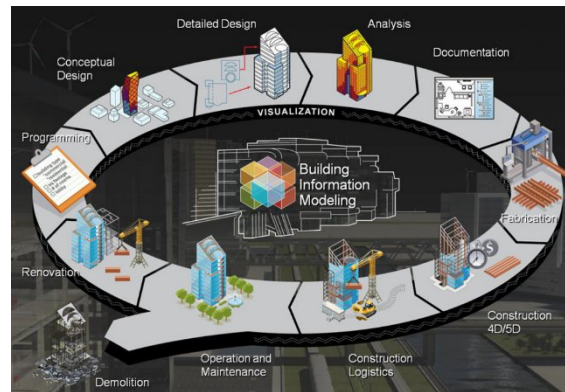
Life cycle of a building, including the use of a BIM model.
